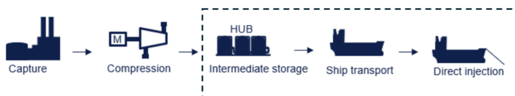
Figure 1: Illustration of the CCS value chain with shipping and offshore direct injection that was included in cost modelling (EPRI, 2025).
