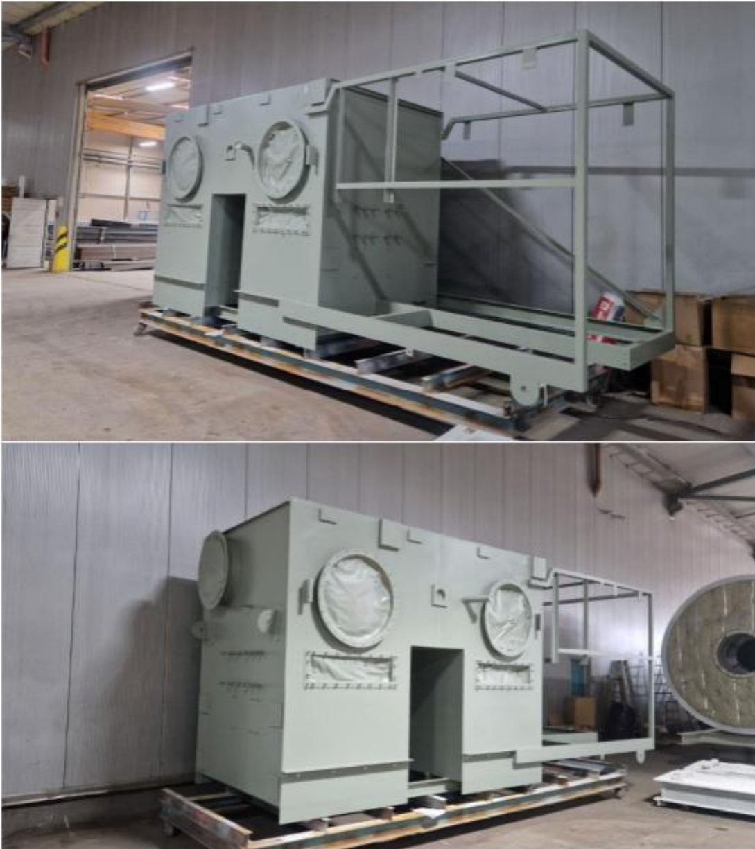
Figure 7: Modified Twin Can (MTC) unit during fabrication
