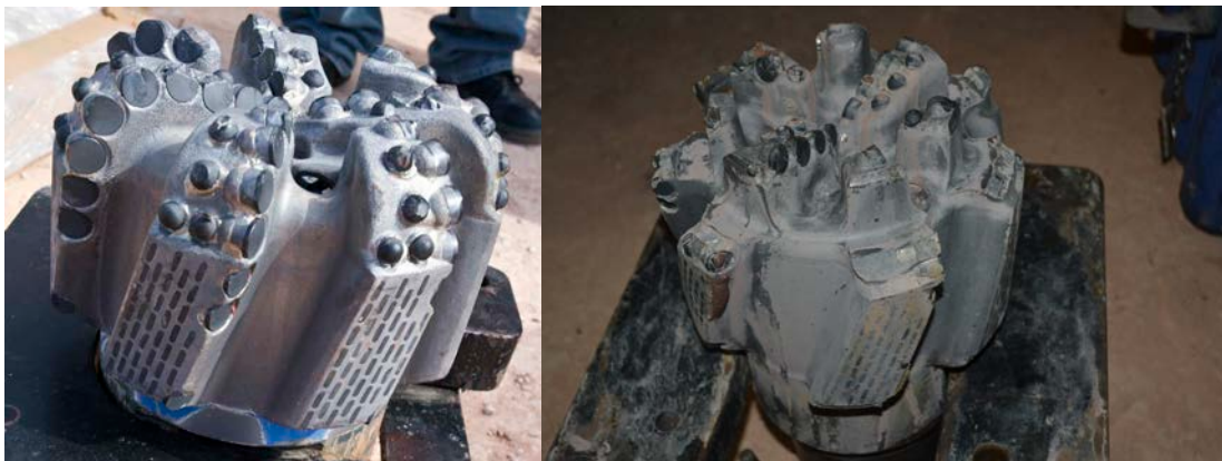
Figure 3. Photos of unused (left) and reamed (right) 7 blade PDC drill bits from Tiltagoonah-1. Photos courtesy of Antonio Ribeiro.
